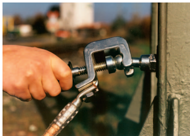
Pic. 13: universal clamp with earthing end synthetic handle
