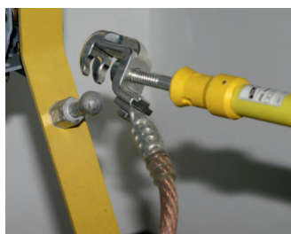
Pic. 3: Earthing stick with universal clamp with cross pin
