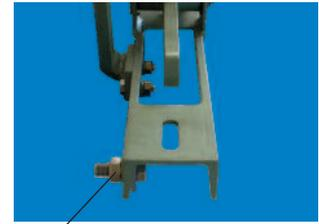
Connector screw for earthing
